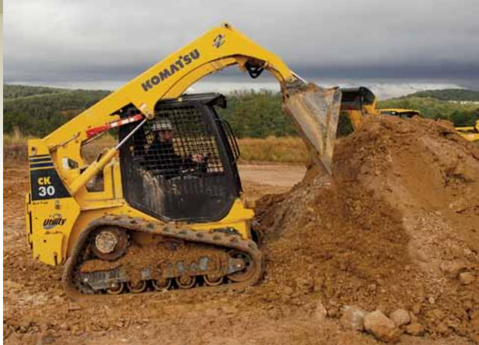
Utility machines, such as the CK30 compact track loader, were required to meet Tier 4 emission standards in 2008. Tier 4 is on the horizon for 175 horsepower and up machines in 2011 and 75 to 175 horsepower must be Tier 4 in 2012.
